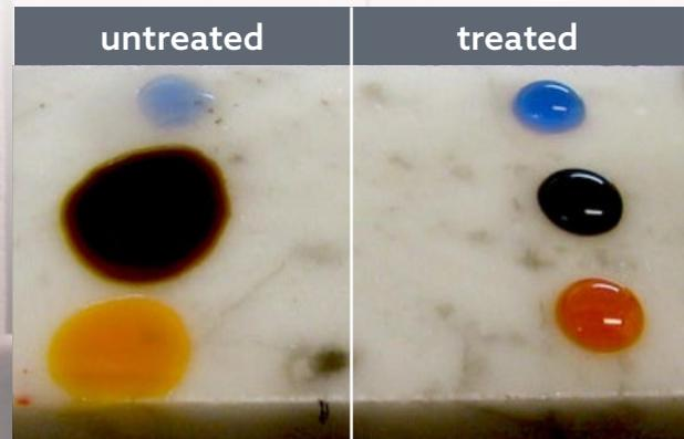
As can be seen above, on the untreated side the wet stains spread and start to penetrate the marble.
