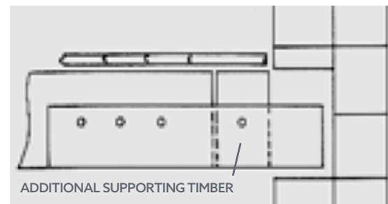
TYPICAL EXAMPLE - 225 mm (9" or up to 430 mm (17") CUTBACKS NECESSARY (NOT TO SCALE)
